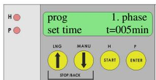
Select the time and temperature with the aid of the ARROW BUTTONS, confirming each value by pressing the ENTER button. Programme the mashing, phases 1-5 and the boiling of the hops. The mode 5 is set to 0 and is only used for special recipes.
