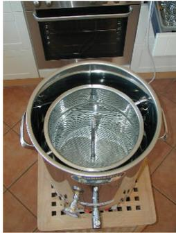
On reaching the mashing temperature, a signal tone sounds, which must be acknowledged by pressing the ENTER button. The malt pipe can now be inserted with the seal facing downwards. Make sure that the pipe is clean, centred and lying flat on the bottom of the boiler. Now insert the first sieve base into the malt pipe and put the first filter cloth on top of it. The cloth must lie on the sheet metal sieve and it is not allowed to float upwards.
