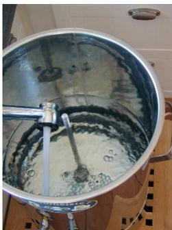
Pour in 53 litres of brewing water – up to about 2 cm below the upper mark on the connecting rod or on the level gauge. Follow the instructions of the brewing controls, and confirm that the Master Brewer has been filled with water by pressing ENTER. The pump ventilates itself automatically and the Master Brewer comes up to the programmed mashing temperature.
