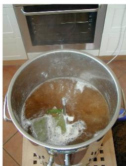
Continue by pressing START in order to start boiling the hops. Avoid over-boiling. Add the first 60g of hops 10 minutes after boiling begins. Do not put on the lid when the hops are boiling either. Steam must be able to escape. Replenish to compensate for the evaporated amount of water or adjust the basic wort. Add the last 30 g of hops 10 minutes before boiling ends.
