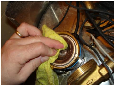
The pump housing should also be carefully cleaned. After this, replace the impeller wheel carefully in the housing.
