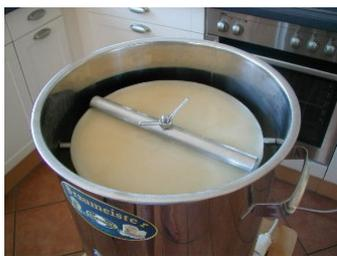
Continue the automatic process by pressing START. Lightly coloured brewing water rises up and runs over. The circulation has begun. The next brewing phases are carried out fully automatically in accordance with the programme. During some brewing phases, the controls initiate a brief pump pause in order to reposition the malt. To display shows the actual and set temperatures, together with the remaining time, which starts to countdown after reaching the set time (flashing).
