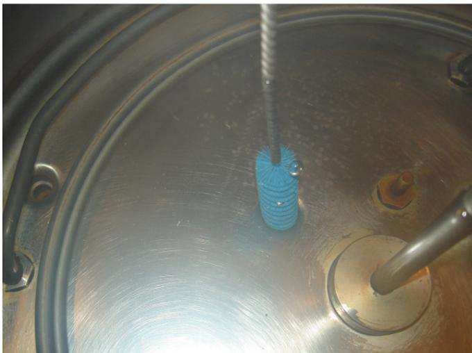
Thorough cleaning includes cleaning out the suction and pressure openings.
