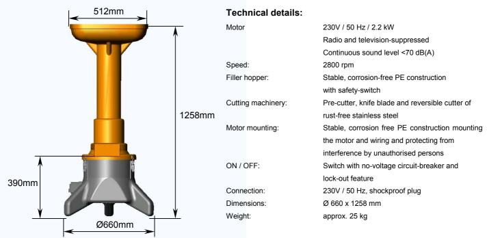
The seed-fruit shredder is supplied ready for operation. It has been designed and manufactured by us in accordance with CE standards, and is exclusively to be used for shredding seed-fruit.
